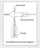
ton an exact pre-defined quantity of CO<sub>2</sub> will be added to the liquid.
