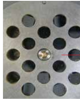
«Harvard» holder with 16 holes and image of microtomed sections of resin-embedded tissues deposited on a 5x5mm silicon square.
