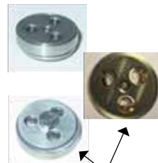
10mm diam. sub-holder for 3 TEM grids. Ref #: 45639345. Correct use: round carbon-film grids on hollow 3mm cylinder, half-grids on plain 3mm cylinder.
