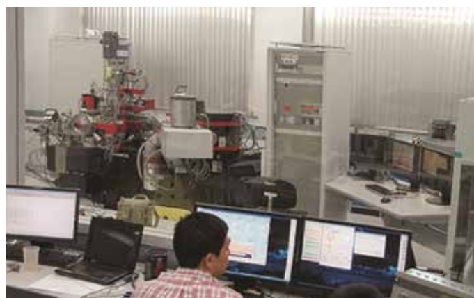
NanoSIMS 50L controlled from a separate room (IGGCAS Beijing, China).
