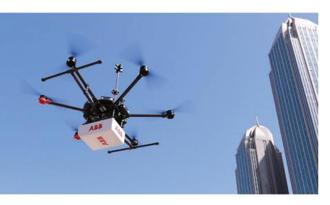
HoverGuard detects natural gas leaks around hard-to-reach sites such as bridges, high-rise buildings, areas with right-of-way restrictions or vegetation coverage, and pipelines.
