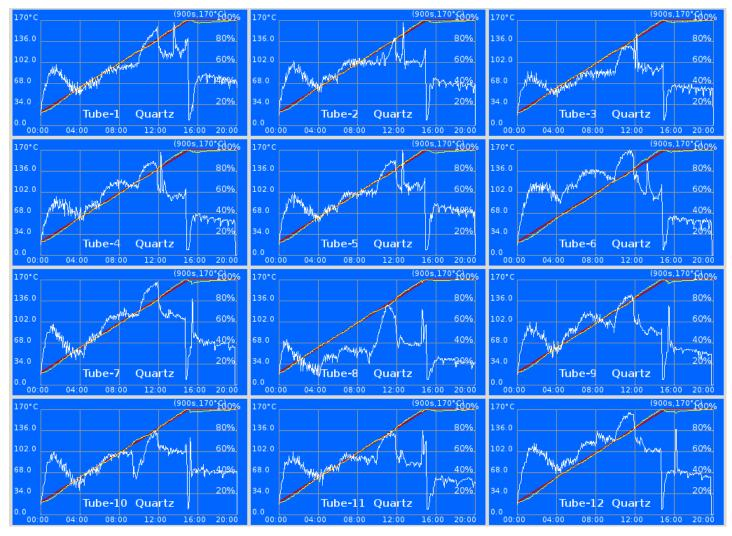
Method: USEPA 3015A; Vessel Type: Quartz; M/V: 0.5 g of Soil, 5 ml HNO, 45 ml Water.
