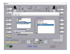
Experimental program setup interface Flexible selection or editing of TPD, TPO, TPR, TPRS, pulse calibration, etc., can set up to 99 programs to achieve full automation of adsorption, desorption, and chemical reactions. The complete experiment setup can be completed within a few minutes.
