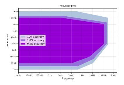
Accuracy contour plot (Based on absolute measurement accuracy)
