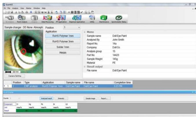
Point Analysis interface, available in various languages, is used for small spot measurements. A live camera display is shown in the window on the left.
